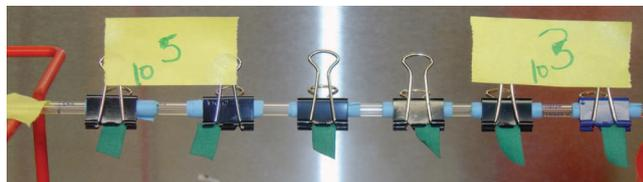
Fig. 2. Air-drying of inoculated scrub coupons after inoculation.
