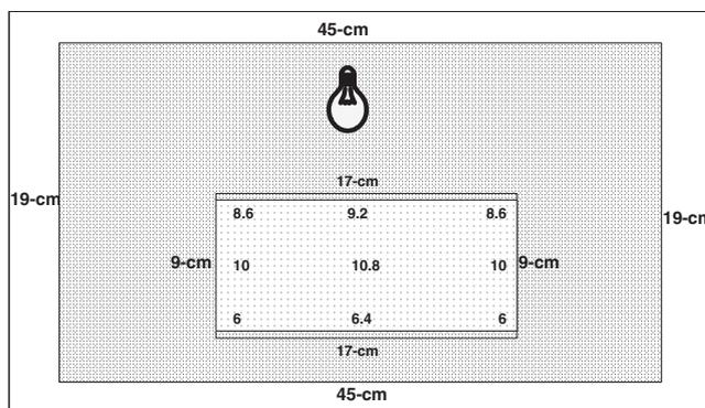
Fig. 3. Diagrammatic sketch of the light box and UVC flux under the lamp (the Petri plate containing the coupons was placed in the center of the lightly shaded area). Numbers indicated in the inner rectangle are flux values (microwatts per square centimeter).
